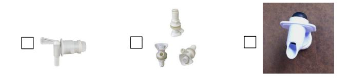
11) Circle the handwashing set up that would be considered acceptable. NOTE: Middle picture from the left has a hands free spigot and third picture from the left has a push button spigot.
